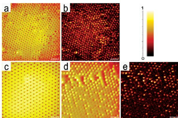
**Figure 2.** Negative ToF-SIMS images (scale bars are 10 μm long). a-b) PST-NH<sub>2</sub> microporous film: (a) sum of all anions; (b)  $m/z$ : 26 (CN<sup>-</sup>). (c–e) PST-NH-bodipy microporous film: (c) sum of all anions before thermal treatment; (d) sum of all anions after 2 h of thermal treatment at 135 °C; (e) same film,  $m/z$ : 19 (F<sup>-</sup>).
