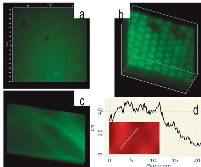
**Figure 5.** PST-NH-bodipy microporous film after heating to  $135 \text{ }^\circ\text{C}$  for 2 h; (a) scanning confocal laser microscopy image; (b, c) 3-D reconstruction of  $z$ -scans done via confocal laser microscopy taken at two different magnifications; (d) roughness analysis measured by AFM along the white line (inset).
