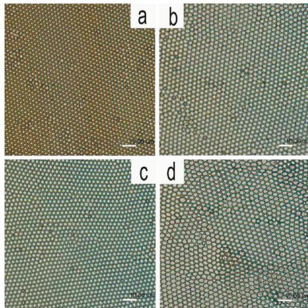
**Figure 3.** Micrographs of thin films prepared by casting 1 mg mL<sup>-1</sup> CS<sub>2</sub> solutions of (a) PST-NH<sub>2</sub>, (b) PST-COOH, (c) PST-OH, (d) PS-PAMS (scale bar is 10 μm long).
