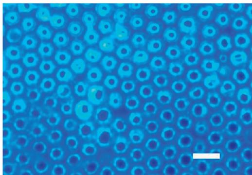
**Figure 1.** Fluorescence microscopy image of a PST-NH<sub>2</sub> honeycomb structured film after treatment with fluorescamine (scale bar is 5 μm long).
