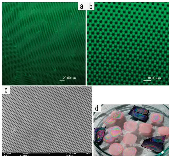
**Figure 4.** (a) PST-NH-bodipy honeycomb structured film;  $330 \mu\text{m}^2$  fluorescence microscopy image with few defects. (b) Bigger magnification of the same film. (c) SEM micrograph of same kind of film. (d) Films prepared by drop-casting a  $\text{CS}_2$  solution of PST-NH-bodipy on glass microscopy coverslips and on silicon wafers.
