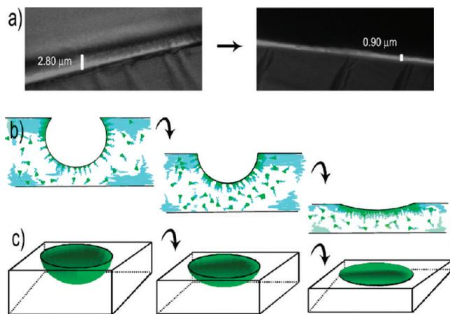
**Figure 6.** Transformation of a PST-NH-bodipy microporous film during thermal treatment (from left to the right). (a) Cross-section of the film placed on silicon substrate. (b) Schemed drawing of the cross-section of a pore. Green triangles stand for the bodipy fluorescent heads of the polymer. (c) 3-D representation of the same phenomenon.
