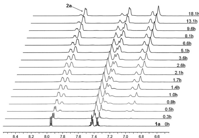
**Figure 1.** Formation of **2a** in CD<sub>3</sub>OD monitored by using <sup>1</sup>H NMR spectroscopy.
