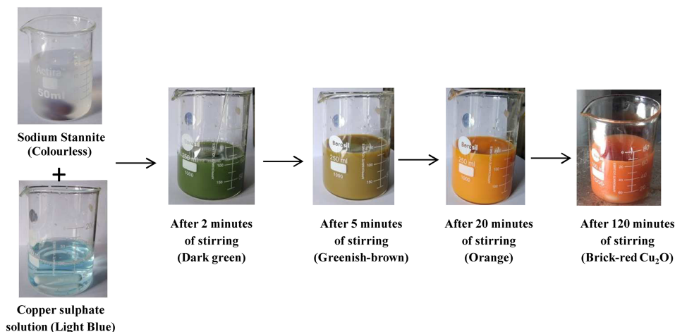
FIGURE 1 Digital images showing the formation of brick-red colored \text{Cu}_2\text{O} materials from \text{CuSO}_4 \cdot 5\text{H}_2\text{O} [Color figure can be viewed at wileyonlinelibrary.com ]
