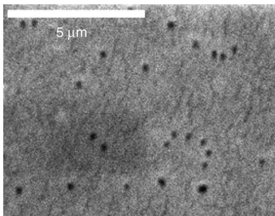
Fig. 1. SEM picture of polycarbonate surface after deposition of gold. The diameter of nanopores in the membranes was 50 nm, and their density was  $3.13 \times 10^5 \text{ mm}^{-2}$ .
