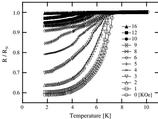
Fig. 4. Temperature dependence of resistance in magnetic fields. Large broadening can be seen below  $T_c$ . Increase of  $H_{c2}(T)$  can also be seen.
