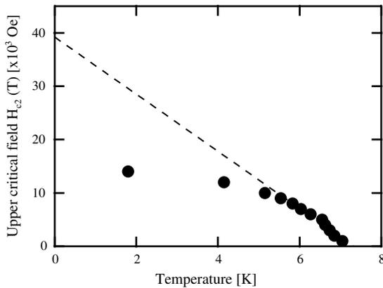
Fig. 6. Magnetic phase diagram of Pb nanowires obtained from magnetic transport measurements. Dots shows the upper critical field  $H_{c2}(T)$  from transport measurements. Dashed line shows the gradient of  $H_{c2}(T)$  obtained from fitting near  $T_c$ .
