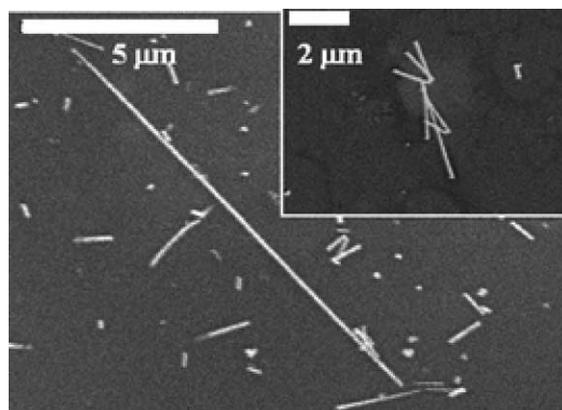
Fig. 2. SEM picture of Pb nanowires and clusters dispersed onto Si substrate after dissolution of polycarbonate membrane. The diameter of nanowires distributes from 80 nm to 100 nm, and the length is longer than 5  $\mu\text{m}$ . The inset shows the nanowires connected with each other by spilled Pb from nanopores. They are connected with each other at the top or bottom by Pb layer made of spilled Pb from nanopores.
