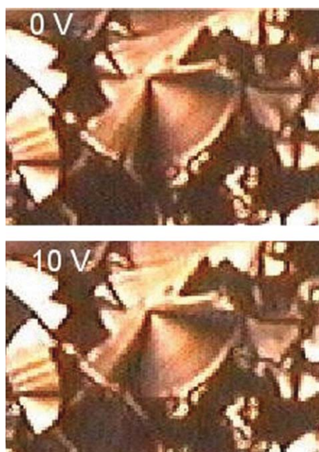
Fig. 4 Changes in the extinction brush direction in a small circular domain in the B 7 -like phase under an electric field (series 1, n = 10 , X = Cl; sample 2 μm thick, 0 V and \sim 10 \text{ V } \mu\text{m}^{-1} ).
