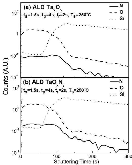
FIG. 1. SIMS profiles of as-deposited (a) ALD  $\text{Ta}_2\text{O}_5$  and (b) ALD  $\text{TaO}_x\text{N}_y$  films using water and  $\text{NH}_4\text{OH}$  as a single source for reactants, respectively.
