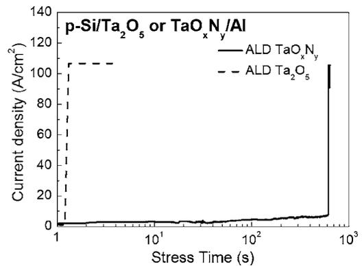
FIG. 5. Time dependent dielectric breakdown data for MOS capacitors with 10 nm ALD  $\text{Ta}_2\text{O}_5$  (solid line) and  $\text{TaO}_x\text{N}_y$  (dotted line) as insulators. The voltage stress measurement was done at an applied voltage of 6.5 MV/cm.
