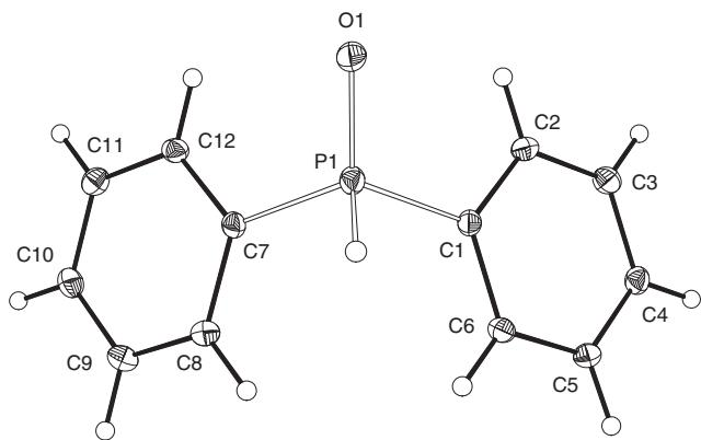
**Fig. 2.** Molecular structure and numbering scheme of diphenylphosphane oxide. The ellipsoids represent a probability of 40 %, H atoms are drawn with arbitrary radii. Selected bond lengths (pm): P1–O1 148.81(11), P1–C1 180.15(14), P1–C7 179.82(15), P1–H1 132.7(18); angles (deg.): O1–P1–C1 113.31(7), O1–P1–C7 113.20(7), O1–P1–H1 116.2(8), C1–P1–C7 108.40(7), C1–P1–H1 101.6(7), C7–P1–H1 102.9(8).
