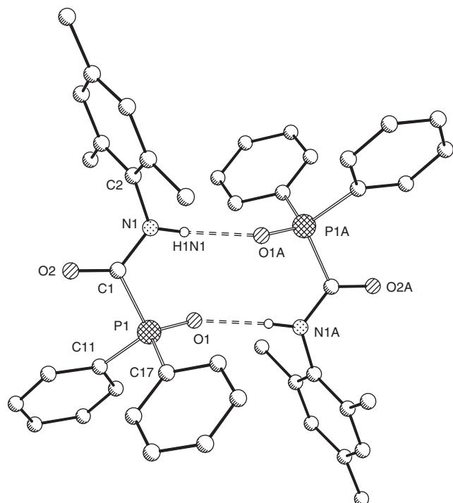
**Fig. 6.** Representative example of the dimerization by  $\text{N}-\text{H}\cdots\text{O}-\text{P}$  hydrogen bridges (dashed line) shown for *N*-mesityl-(diphenylphosphoryl)-formamide (**6**). All atoms are shown with arbitrary radii, carbon-bound hydrogen atoms are neglected for clarity reasons.
