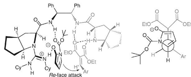
**Scheme 3** Proposed activation model for asymmetric VM reaction catalyzed by **2**.
