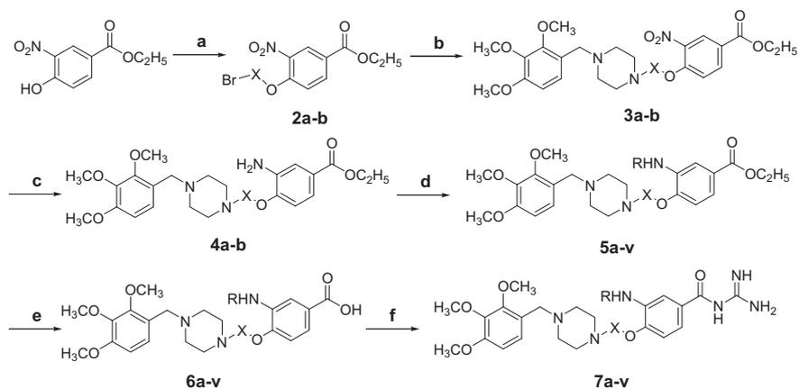
**Scheme 1.** Reagents and conditions: (a) 1,2-dibromo ethane/1,3-dibromo propane,  $K_2CO_3$ ,  $CH_3CN$ , reflux; (b) trimetazidine,  $K_2CO_3$ ,  $CH_3CN$ , 20–80 °C; (c)  $Fe/HCl/50\%$  (v/v) ethanol, reflux; (d)  $CH_2Cl_2/Et_3N$ , 0–5 °C; (e) methanol/ $K_2CO_3$ , reflux; (f) guanidine/HOBT/EDCI/DMF, room temperature.
