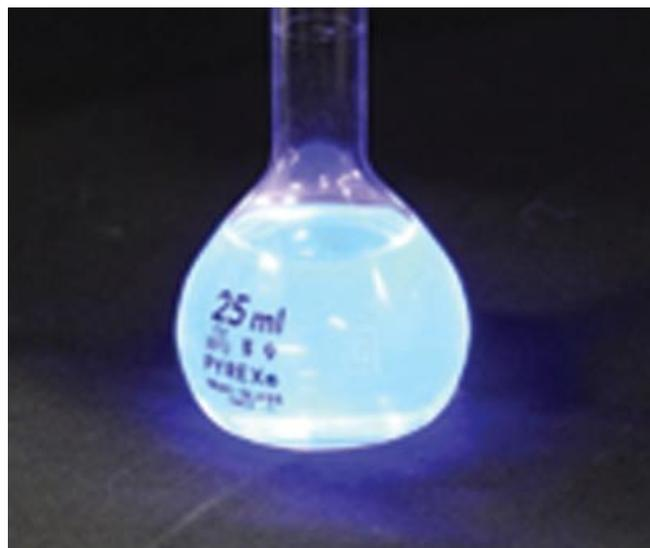
FIGURE 2 Emission from a chloroform solution of **DTSP2-Au** excited at 364 nm.
