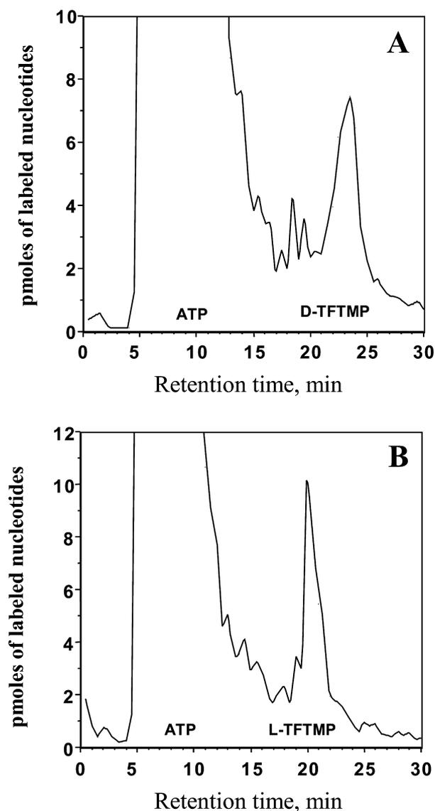
**Figure 3.** Phosphorylation of TFT and L-TFT by HSV-1 TK. HPLC elution profiles of the reaction products of TFT (panel A) and L-TFT (panel B) after 60 min incubation with HSV-1 TK and [<sup>32</sup>P]-ATP.
