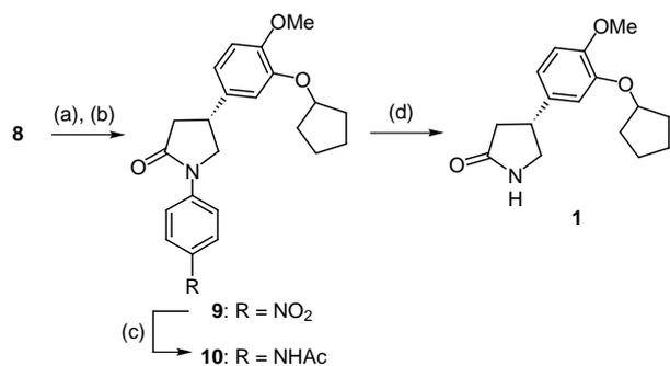
Reagents and conditions: (a) NaCl, aq. DMSO, 160 °C, 2 h, 97%; (b) recrystallization 71%; (c) Fe, AcOH, reflux, 2 h, 86%; (d)  $\text{Ce}(\text{NH}_4)_2(\text{NO}_2)_6$  (2.5 eq), aq. MeCN, 0 °C, 1 h, 71%.
