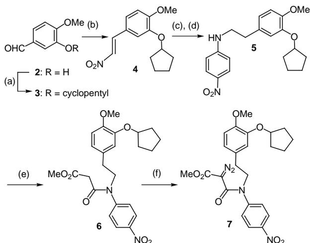
**Reagents and conditions:** (a) cyclopentyl bromide,  $K_2CO_3$ , DMF, 60 °C, 12 h, 91%; (b)  $MeNO_2$ ,  $NH_4OAc$ , reflux, 3 h, 79%; (c)  $LiAlH_4$ , THF, reflux, 1.5 h; (d) 4-fluoronitrobenzene,  $Na_2CO_3$ , EtOH, sealed tube, 150 °C, 12 h, 60% (2 steps); (e)  $MeO_2CCH_2COCl$ ,  $Me_2NC_6H_5$ ,  $CH_2Cl_2$ , 0 °C, 2 h, 97%; (f) 4-acetamidobenzenesulfonyl azide, DBU, MeCN, 0 °C, 3 h, 91%.
