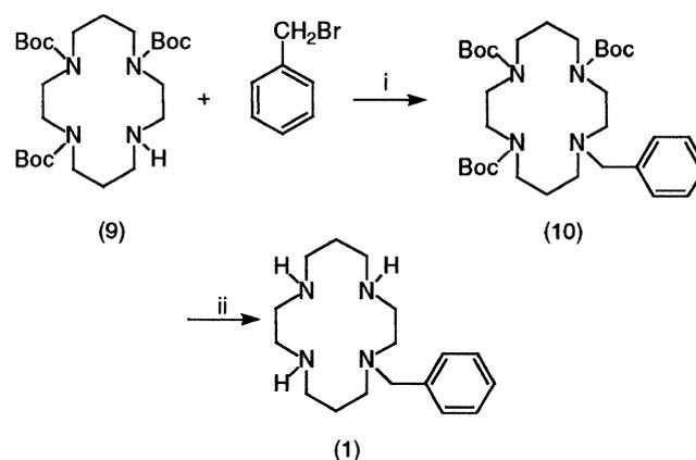
**Scheme 1.** Boc = tert-butoxycarbonyl. Reagents and conditions: (i) Cs<sub>2</sub>CO<sub>3</sub>, dry CH<sub>3</sub>CN, reflux; (ii) 3 M HCl–MeOH.
