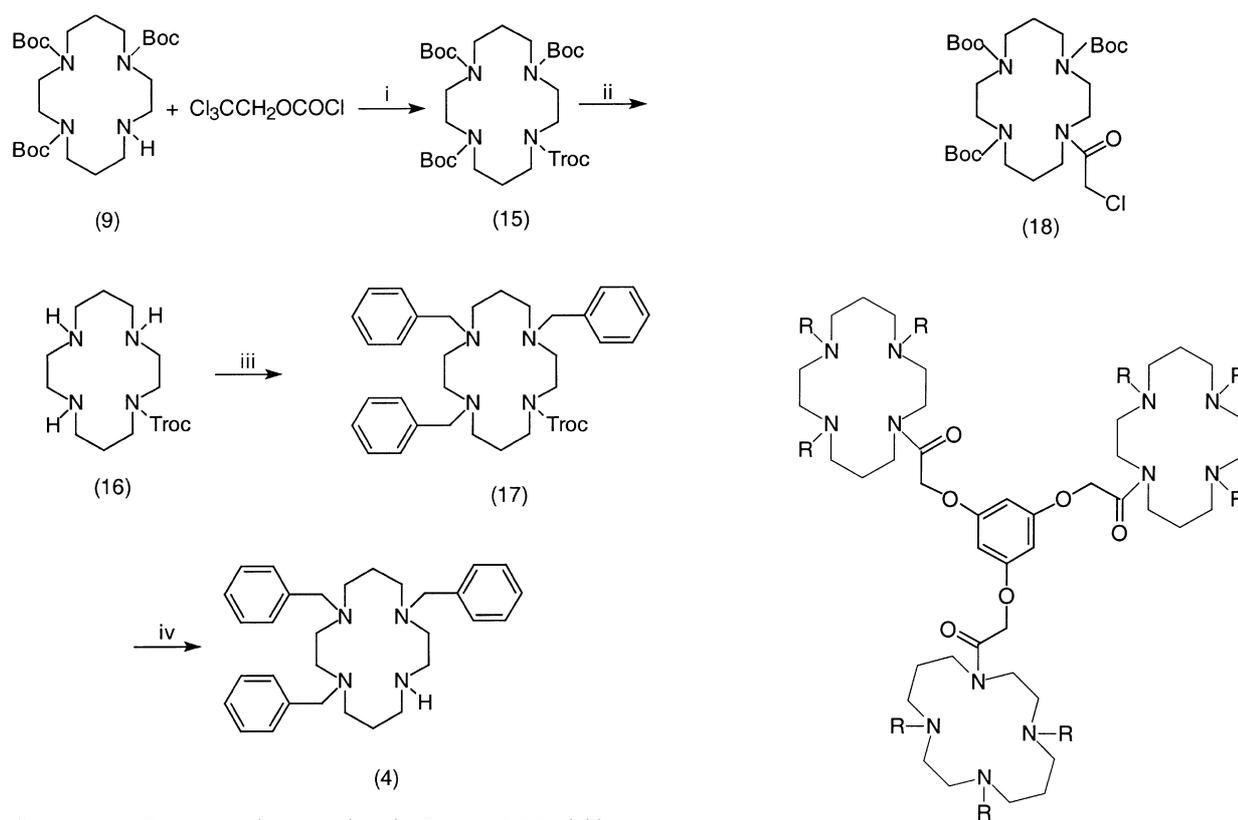
**Scheme 3.** Boc = tert-butoxycarbonyl; Troc = 2,2,2-trichloroethoxycarbonyl. *Reagents and conditions:* (i) Et<sub>3</sub>N, dry CH<sub>2</sub>Cl<sub>2</sub>; (ii) 3 M HCl–MeOH; (iii) PhCH<sub>2</sub>Br, Cs<sub>2</sub>CO<sub>3</sub>, dry CH<sub>3</sub>CN, reflux; (iv) Zn, HOAc.
