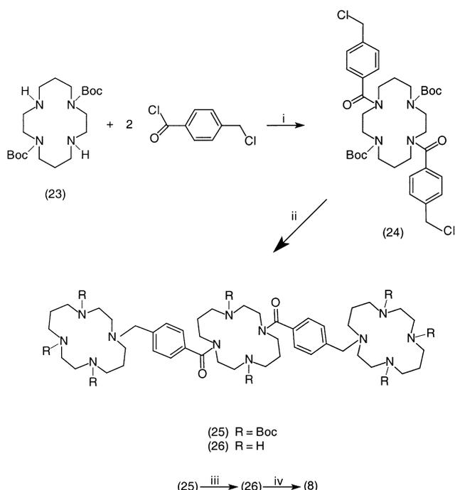
**Scheme 6.** Boc = tert-butoxycarbonyl. *Reagents and conditions:* (i) Et<sub>3</sub>N, dichloromethane; (ii) Compound (9), Cs<sub>2</sub>CO<sub>3</sub>, KI, CH<sub>3</sub>CN; (iii) 3M HCl–MeOH; (iv)  $BH_3 \cdot Me_2S$ , then MeOH/H<sub>2</sub>O/conc. HCl (20 : 10 : 10).
