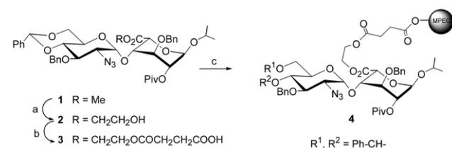
Scheme 2 a) Ethylene glycol, Bu<sub>2</sub>SnO, toluene, 135 °C, 81%; b) succinic anhydride, DMAP, Py, 98%; c) MPEG, DIC, DMAP, CH<sub>2</sub>Cl<sub>2</sub>, 100%.
