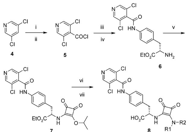
**Scheme 1.** (i) LDA, THF,  $-78^{\circ}\text{C}$ , 30 min then CO<sub>2</sub>; (ii) SOCl<sub>2</sub>, DCM; (iii)  $\alpha$ -N-Boc 4-aminophenylalanine ethyl ester, *N*-methyl morpholine, DCM; (iv) 3 M HCl in EtOAc; (v) 3,4-diisopropoxy-3-cyclobuten-1,2-dione, DIPEA, EtOH; (vi) R<sub>1</sub>R<sub>2</sub>NH, EtOH; (vii) LiOH, THF, H<sub>2</sub>O.
