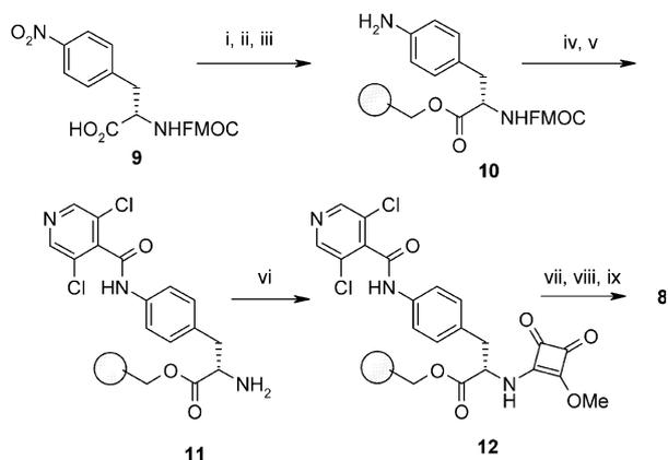
**Scheme 2.** (i) Paramax Wang resin, 2,6-dichlorobenzoyl chloride, pyridine, DMF; (ii) 20% acetic anhydride, DMF; (iii) SnCl<sub>2</sub>(H<sub>2</sub>O)<sub>2</sub>, DMF; (iv) **5**, DIPEA, DCM; (v) 20% piperidine, DMF; (vi) 3,4-dimethoxy-3-cyclobuten-1,2-dione, DMF,  $70^{\circ}\text{C}$ ; (vii) R<sub>1</sub>R<sub>2</sub>NH, DCM; (viii) 60% TFA, DCM; (ix) HPLC purification.
