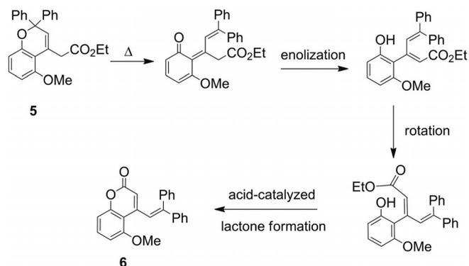
Scheme 5. Mechanism for the formation of **6**.
