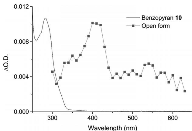
Figure 2. Normalised absorption spectra of **10** in  $10^{-4}$  M degassed acetonitrile, collected before and after laser irradiation at 266 nm.
