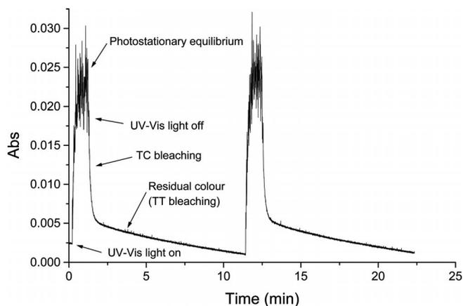
Figure 1. Absorbance evolution during UV/Vis irradiation and darkness for 2,2-diphenyl-2*H*-chromene.
