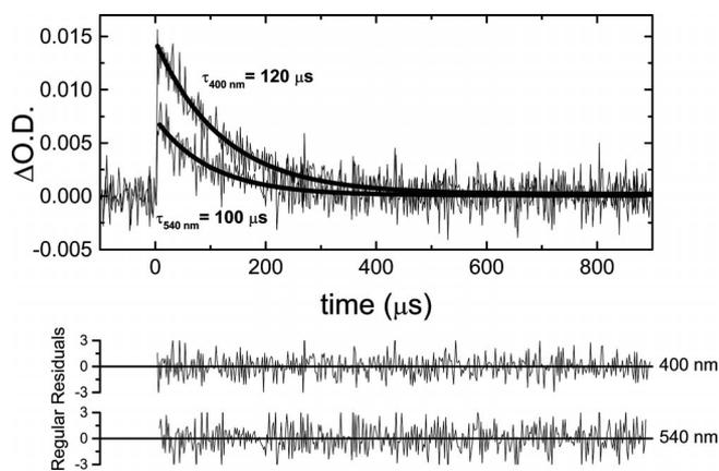
Figure 3. Decay traces for the open form of **10** in MeCN collected at 400 and 540 nm. Also shown are the monoexponential fittings to the decays and the corresponding residuals distribution.
