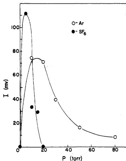
**Figure 2.** The effects of Ar and  $\text{SF}_6$  on HF laser intensity. Mixtures (3 Torr) of 1:2  $\text{CF}_3\text{C}_2\text{H}:\text{NO}_2$  and 5 Torr mixtures of 1:4  $\text{CF}_3\text{C}_2\text{H}:\text{NO}_2$  were diluted with Ar and  $\text{SF}_6$ , respectively. Flash energy was maintained constant at 1.6 kJ.
