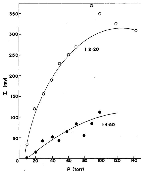
**Figure 3.** Total pressure dependence of HF laser emission for 1:2:20 and 1:4:50  $\text{CF}_3\text{C}_2\text{H}:\text{NO}_2:\text{Ar}$  mixtures. Flash energy 1.6 kJ.
