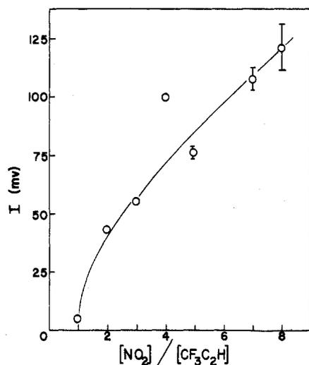
**Figure 1.** HF laser intensity as a function of  $[\text{NO}_2]/[\text{CF}_3\text{C}_2\text{H}]$  ratio.  $\text{CF}_3\text{C}_2\text{H}$  (1 Torr) was added to varying amounts of  $\text{NO}_2$  and Ar to make a total pressure of 60 Torr, flashed with 1.6-kJ energy.
