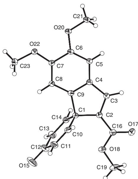
**Fig. 5.** Molecular structure of compound **54** ( $C_{18}H_{16}O_5$ ) with labeling of selected atoms. Anisotropic displacement ellipsoids show 30% probability levels. Hydrogen atoms are drawn as circles with small radii.
