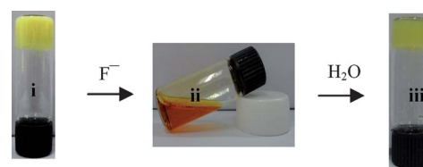
Fig. 11 Photographs of (i) organogel formed from compound IV in THF, (ii) after addition of TBAF (1 equiv.), and (iii) after addition of water (0.2 ml).
