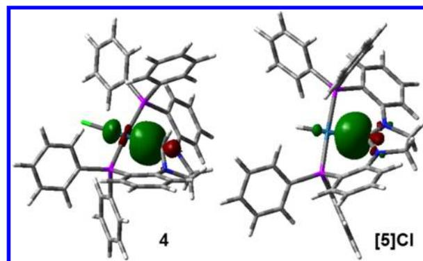
**Figure 4.** Pictorial representations of the Pt–C natural bond orbitals computed for complexes **4** and [5]Cl. NBO of **4**: 35.6% Pt, 64.4% C (26.6% s/73.4% p). NBO of [5]Cl: 23.4% Pt, 76.6% C (43.7% s/56.3% p).
