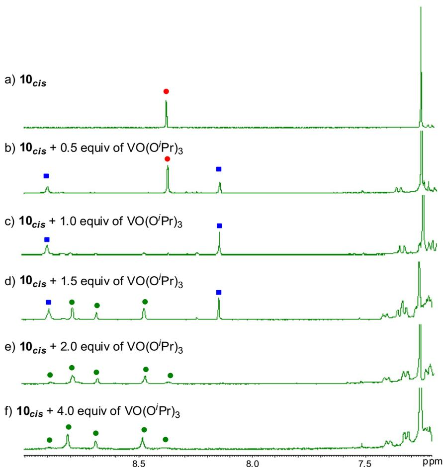
**Figure 1.**  $^1\text{H}$  NMR spectra for the complexation of  $\mathbf{10}_{cis}$  with  $\text{VO}(\text{O}^i\text{Pr})_3$ . Each reaction was carried out in ethanol/dichloromethane at room temperature for 1 h under argon. Then, the solvent was replaced by  $\text{CDCl}_3/\text{CD}_3\text{OD}$  (20:1) for the  $^1\text{H}$  NMR study.
