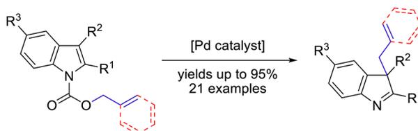
A set of general methods for the palladium-catalyzed decarboxylative C<sup>3</sup>-allylation and C<sup>3</sup>-benzylation of indoles, starting from the corresponding *N*-alloc and *N*-Cbz indoles, respectively, is reported. This chemistry provides ready access to a wide range of functionalized indolenines in good to excellent yields. A tandem process, wherein the palladium catalyzed allylation chemistry is coupled with a Mizoroki–Heck reaction, offers a simple route to cinnamylated products.
