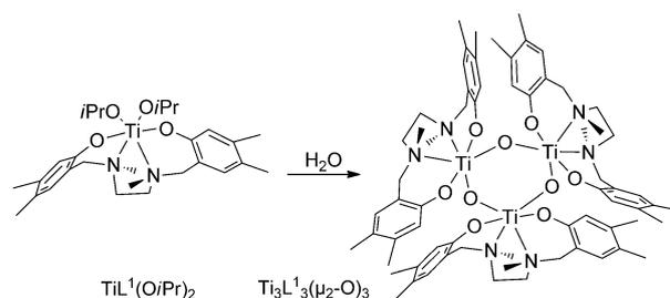
**Scheme 1.** Salan complex TiL<sup>1</sup>(OiPr)<sub>2</sub> and its trinuclear hydrolysis product Ti<sub>3</sub>L<sub>3</sub>(μ<sub>2</sub>-O)<sub>3</sub>.
