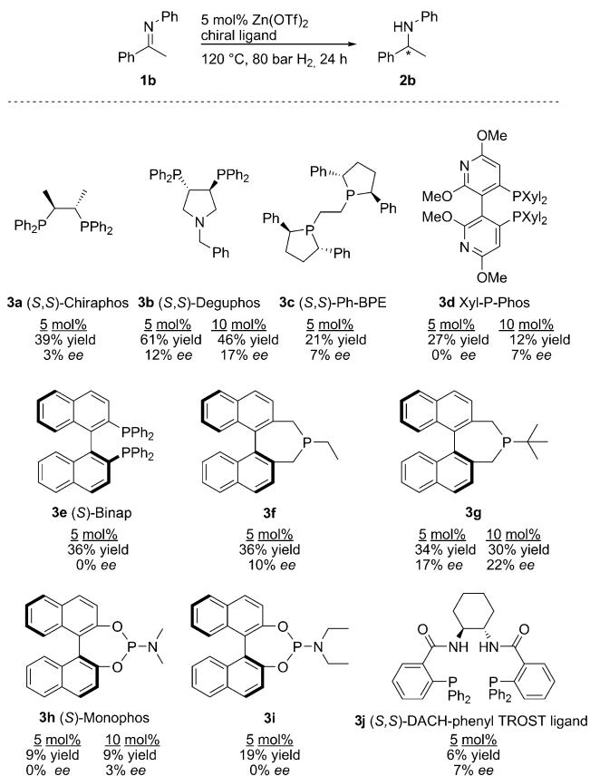
Figure 2. Zn-catalyzed hydrogenation of **1b** in the presence of different chiral P-containing ligands **3** (GC yields are presented).
