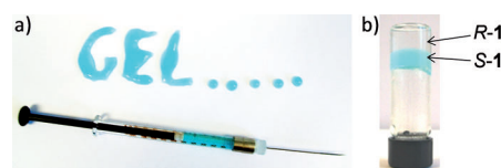
Figure 13. Demonstration of the application of chiral hydrogels of compound 1 as an injectable material. a) A solution of the gelator is charged into the syringe at 50 °C and a gel forms quickly after depositing the solution onto a surface at room temperature. b) Gels of compounds R -1 and S -1 can be easily prepared in the same vial by the consecutive addition of warm solutions of the gelator into the vial at room temperature. The blue color is due to the addition of methylene blue.
