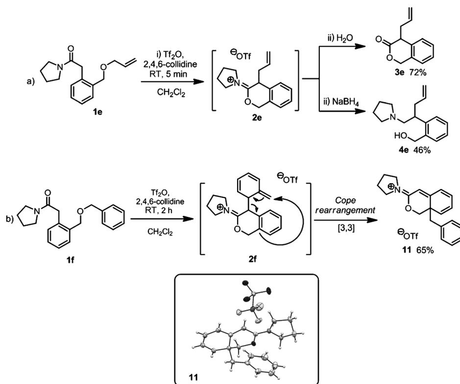
Scheme 5. Claisen–Cope rearrangement of **1f** to produce iminium ether **11**. An ORTEP drawing of **11**-OTf is shown, ellipsoids are presented at the 50% probability level.
