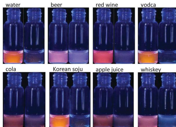
**Fig. 3** Pictures of beverage samples with and without GHB containing **GHB Orange** under irradiation using a hand-held 365 nm lamp. (final concentrations: DMSO 50% by volume, **GHB Orange** 50  $\mu\text{M}$ , GHB 5  $\text{mg mL}^{-1}$ ).
