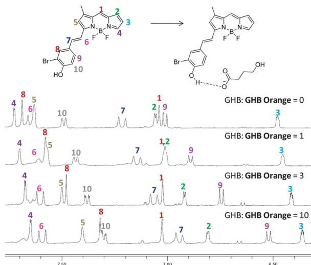
**Fig. 4** Partial  $^1\text{H}$  NMR spectra of **GHB Orange** (30 mM) upon addition of different equivalents of GHB in DMSO- $d_6$  and  $\text{D}_2\text{O}$  (9 : 1).
