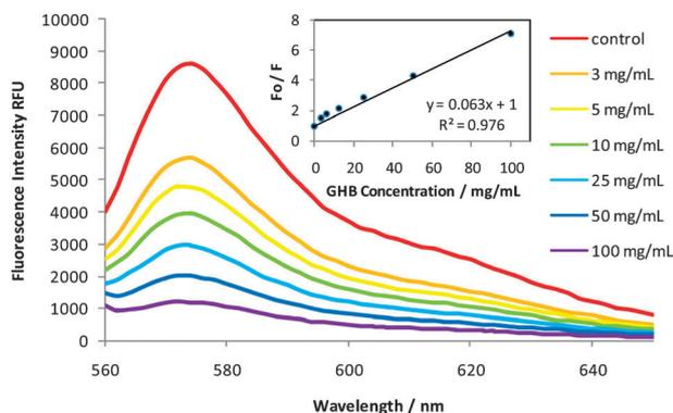
**Fig. 2** Fluorescent spectra of **GHB Orange** (20  $\mu\text{M}$ ) after incubation with different concentrations of GHB. (inner) Linear correlation of fold change of fluorescence versus concentration of GHB.
