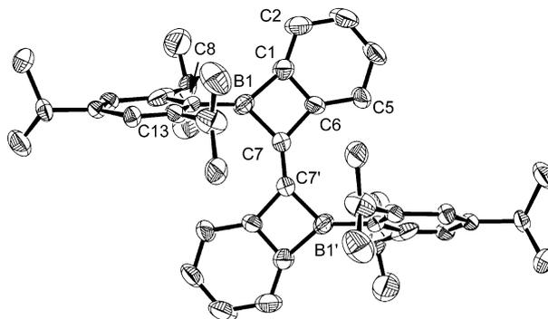
**Figure 1.** Thermal ellipsoid (50%) diagrams of the molecular structure of **2**. Selected bond lengths [Å], angles [°], and dihedral angles [°]: C1–B1 1.575(5), C7–C7' 1.330(7), C7–C6 1.485(5), C1–C6 1.416(5), C7–B1 1.581(5), C1–B1–C7 86.6(3), C1–B1–C8 138.3(3), C7–B1–C8 134.2(3), C13–C8–B1–C7 67.6(6), C1–C6–C7–C7' 179.7(2).
