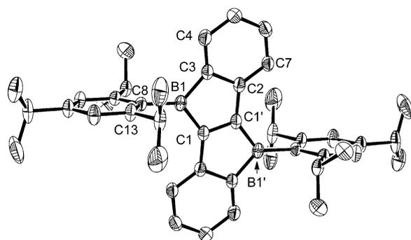
**Figure 3.** Thermal ellipsoid (50%) diagrams of the molecular structure of **3**. Selected bond lengths [ $\text{\AA}$ ], angles [ $^\circ$ ], and dihedral angles [ $^\circ$ ]:  $\text{C1-B1}$  1.571(4),  $\text{C1-C1'}$  1.367(5),  $\text{C1'-C2}$  1.480(4),  $\text{C2-C3}$  1.419(3),  $\text{C3-B1}$  1.588(4),  $\text{C3-B1-C1}$   $102.1(2)$ ,  $\text{C8-B1-C1}$   $128.6(2)$ ,  $\text{C8-B1-C3}$   $129.2(2)$ ,  $\text{C1-B1-C8-C13}$   $-90.1(4)$ ,  $\text{C1-C1'-C2-C3}$   $0.1(4)$ .
