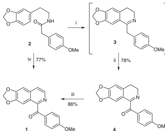
**Scheme 1** Reagents and conditions: (i) POCl<sub>3</sub>, benzene, 80 °C, 2 h; (ii) DBU, CH<sub>2</sub>Cl<sub>2</sub>, r.t., 2 h, 78%; (iii) DBU, CH<sub>2</sub>Cl<sub>2</sub>, r.t., 24 h, 86%; (iv) POCl<sub>3</sub>, benzene, 80 °C, 2 h, then DBU, CH<sub>2</sub>Cl<sub>2</sub>, r.t., 24 h, 77%.
