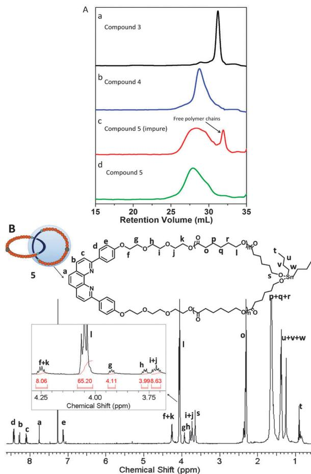
**Fig. 1** (A) GPC curves for the (a) catenane initiator **3**, (b) catenated polymer with complex **4**, (c) decomplexation product of catenated polymer **5**, and (d) purified catenated polymer **5**. (B) <sup>1</sup>H NMR spectrum of purified catenated polymer **5**.
