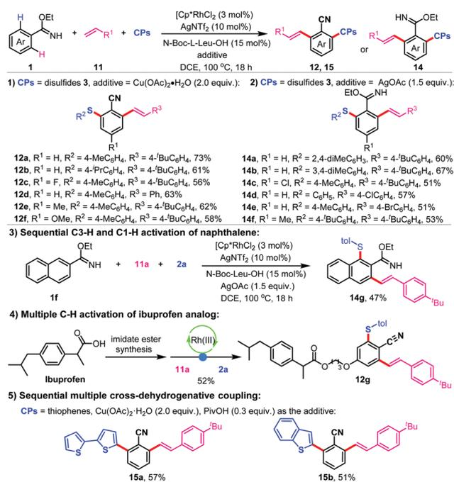
Scheme 5 Sequential multiple C-H activation. Conditions: **1** (0.3 mmol), **11** (0.45 mmol), **CPs** (0.45 mmol), [Cp\*RhCl<sub>2</sub>]<sub>2</sub> (3 mol%), AgNTf<sub>2</sub> (10 mol%), Cu(OAc)<sub>2</sub>·H<sub>2</sub>O (2.0 equiv.), DCE (1 mL), 100 °C, 18 h.
