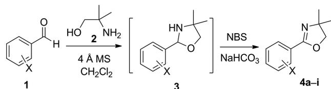
Scheme 1. Preparation of halophenyl-2-oxazolines **4a–4i** from aldehydes **1** (MS = molecular sieves).
