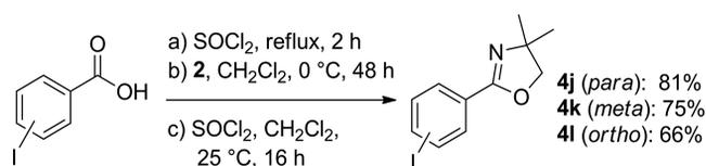
Scheme 2. Preparation of halophenyl-2-oxazolines **4j–4l** from carboxylic acid.
