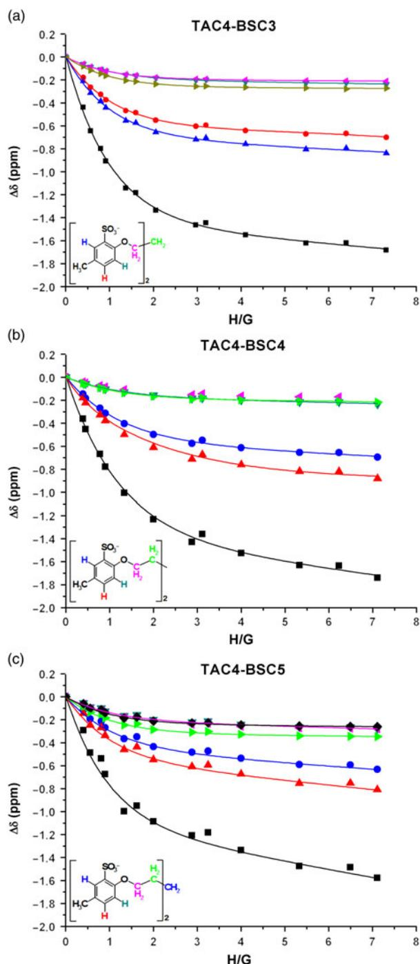
Figure 1. (Colour online) CIS diagrams for the **BSC<sub>n</sub>–TAC4** systems ( $n = 3, 4, 5$  for (a), (b) and (c), respectively) in  $D_2O$ , pD 7.1, 27°C.  $C_{BSCn} = 2.5 \times 10^{-4} \text{ mol dm}^{-3}$ .
