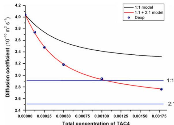
Figure 5. (Colour online) BSC3 self-diffusion coefficients in D<sub>2</sub>O at pD 7.1, 27°C. Blue full circles; experimental data points; black line; curve predicted for the HG model; red line; curve predicted for the HG + H<sub>2</sub>G model. Blue lines indicate the expected diffusion value for HG and H<sub>2</sub>G, respectively.  $C_{\text{BSC}n} = 2.5 \times 10^{-4} \text{ mol dm}^{-3}$ .
