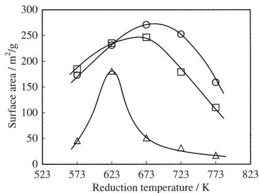
**Figure 2.** Effect of reduction temperature on the surface areas of H<sub>1.55</sub>MoO<sub>3</sub> (○), MoO<sub>3</sub> (△), and Pt/MoO<sub>3</sub> (□). Reduction period: 12 h.
