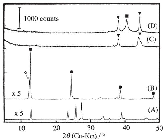
**Figure 1.** XRD patterns of MoO<sub>3</sub> and H<sub>x</sub>MoO<sub>3</sub>. (A), MoO<sub>3</sub>; (B), H<sub>x</sub>MoO<sub>3</sub>; (C), (B) reduced at 573 K for 12 h; (D), (B) reduced at 773 K for 12 h. (●), H<sub>1.68</sub>MoO<sub>3</sub>; (▼), MoO<sub>x</sub>H<sub>y</sub>; (■), Mo metal; (◇), unknown.
