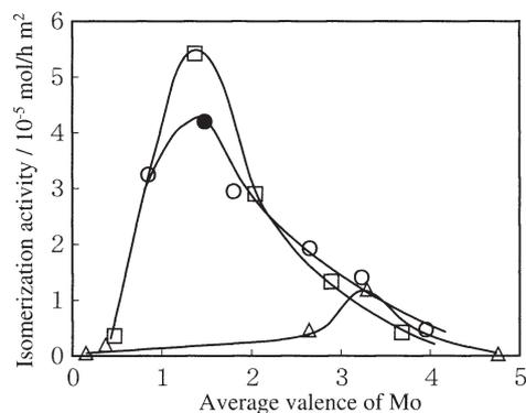
**Figure 3.** Relationship between the pentane isomerization activity and the average valence of Mo. H<sub>1.55</sub>MoO<sub>3</sub> (○), MoO<sub>3</sub> (△), and Pt/MoO<sub>3</sub> (□) were reduced at 573–773 K for 12 h. H<sub>1.55</sub>MoO<sub>3</sub> (●) was reduced at 773 K for 6 h. Reaction conditions: temperature, 523 K; H<sub>2</sub>/C<sub>5</sub>, 10; W/F, 10 g-cat./h mol.
