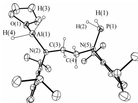
Figure 4. Molecular structure of **6g**·THF; H atoms in the Dipp substituents omitted for clarity; 50% probability ellipsoids. Selected distances [Å]: P(1)–H(1) 1.33(3), P(1)–H(2) 1.36(3), P(1)–N(5) 1.685(2), C(3)–C(4) 1.522(4), N(2)–Al(1) 1.813(2), Al(1)–H(3) 1.51(3), Al(1)–H(4) 1.53(3), Al(1)–O(1) 1.916(2).
