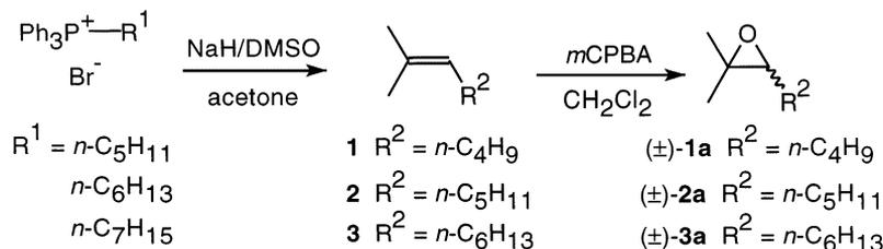
**Scheme 1.** Synthesis of substrates  $(\pm)\text{-1a–3a}$ .
