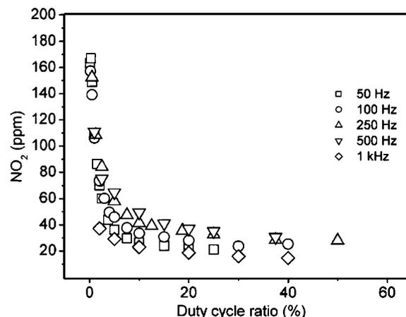
FIG. 3. Influence of the duty cycle ratio, DCR, on the formation of NO<sub>2</sub> for different pulse repetition rates. Labels identical to Fig. 2.
