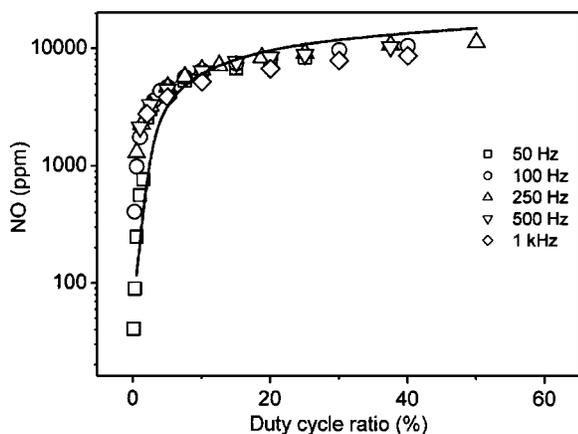
FIG. 2. Influence of the duty cycle ratio, DCR, on the formation of NO for different pulse repetition rates. Peak current 80 mA, 4 mbar, dry air, 20 scem. The solid line is the computed results from numerical code.
