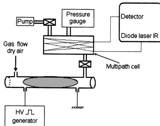
FIG. 1. Experimental set up: pulsed dc discharge, the infrared laser TOBI and the multipath cell.
