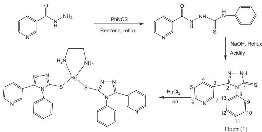
**Scheme 1.** Preparation of the ligand Hpptt (**1**) and its complex [Hg(en)(4-pptt)<sub>2</sub>] (**2**).
