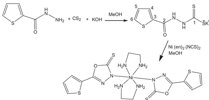
**Scheme 3.** Preparation of  $[\text{Ni}(\text{en})_2(5\text{-thot})_2]$  (**4**).
