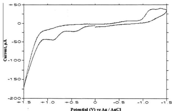
Fig. 1. Cyclic voltammogram of  $[\text{Ni}(\text{en})_2(5\text{-thot})_2]$  in DMSO at PGE using 0.2 M KCl as the supporting electrolyte.
