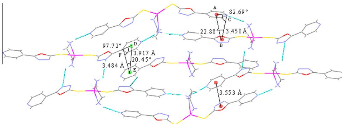
Fig. 10. Showing  $\pi \cdots \pi$  stacking and the relative shift between two pyridine–pyridine and pyridine–oxadiazole ring centroids.
