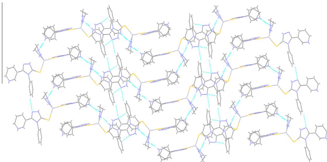
Fig. 7. N–H...N interaction between the pyridine nitrogen and NH<sub>2</sub> of an en molecule.
