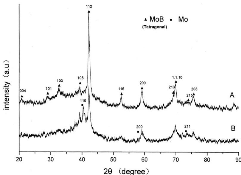
Fig. 2. The patterns of XRD of the samples annealed for 2 h at  $900^\circ\text{C}$ : (A) annealing sample 8 at  $900^\circ\text{C}$ ; (B) annealing sample 6 at  $900^\circ\text{C}$ .
