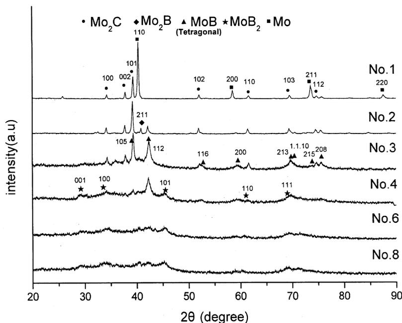
Fig. 1. The patterns of XRD of as-synthesized samples prepared under the condition of different molar ratio of  $\text{KBH}_4$  to  $\text{MoO}_3$ .
