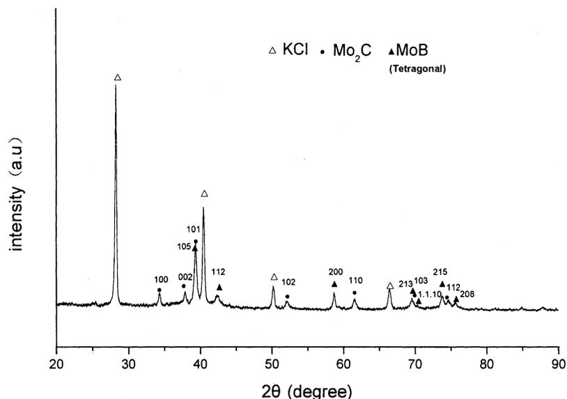
Fig. 5. The pattern of XRD of the mixture of sample produced by the reaction of  $\text{MoO}_3$ ,  $\text{KBH}_4$ , and  $\text{CCl}_4$  with 1:3.5:1.82 as the molar ratio between  $\text{MoO}_3$ ,  $\text{KBH}_4$ , and  $\text{CCl}_4$ .
