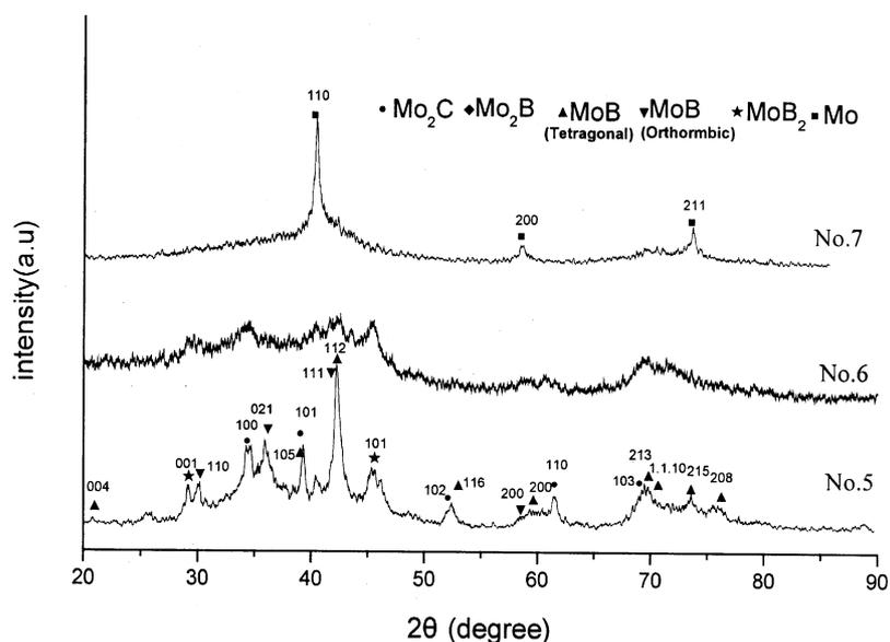
Fig. 3. The patterns of XRD of the samples prepared under the condition of different molar ratio of  $\text{CCl}_4$  to  $\text{KBH}_4$ .
