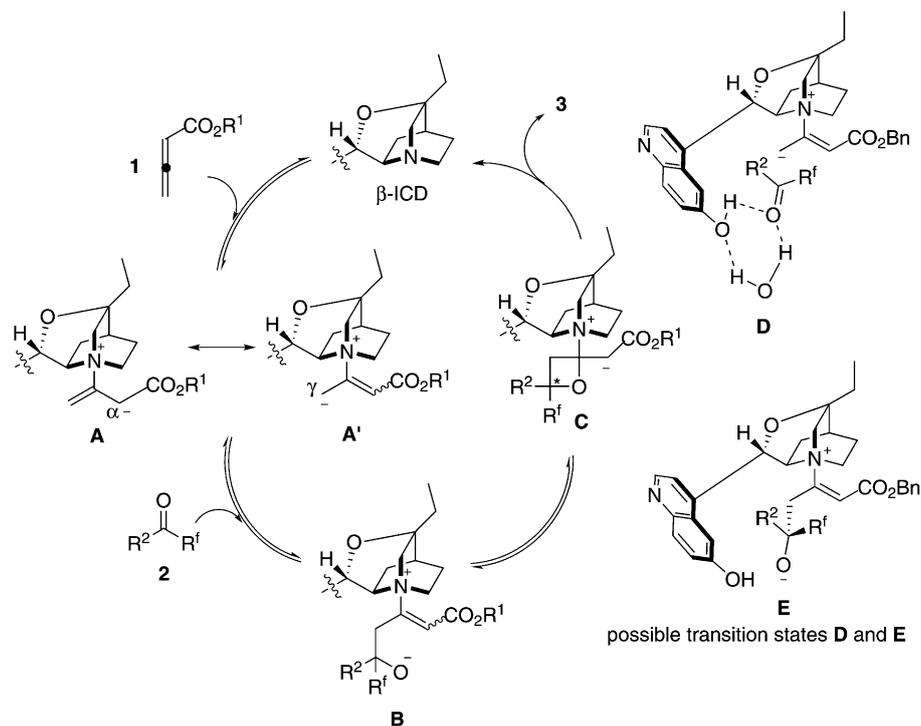
**Scheme 2.** A plausible catalytic cycle for the asymmetric [2+2] annulation.
