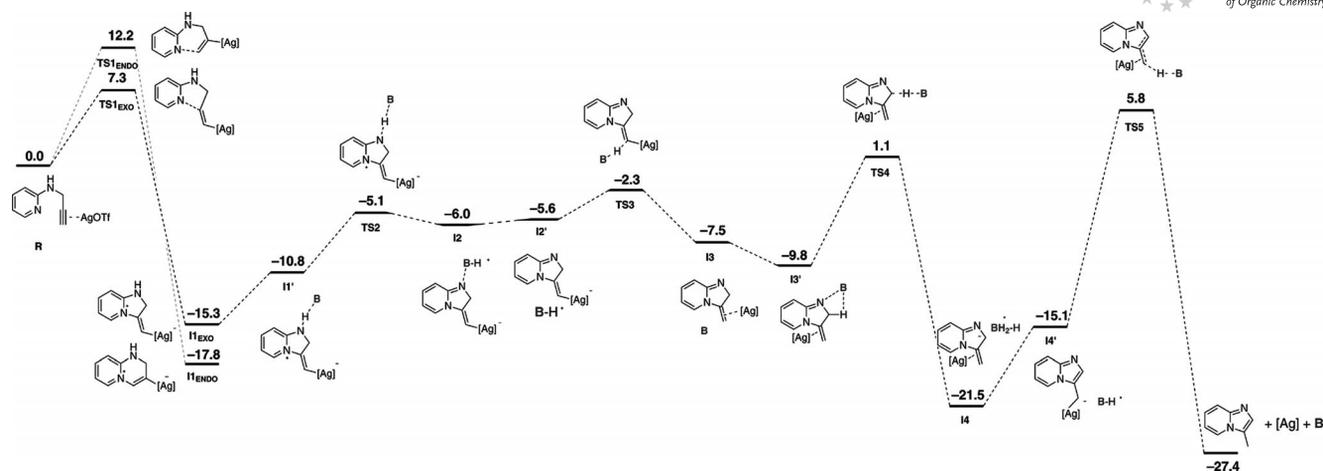
Figure 1. Free-energy profile (in kcal/mol) computed in solution (acetonitrile) for the Ag-catalyzed heterocyclization of **1a**. **B** refers to **1a** acting as a base assisting the proton-shift steps.
