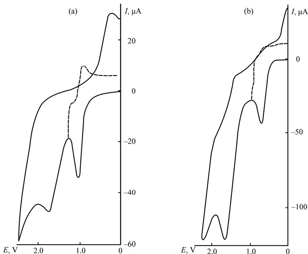
**Fig. 1.** Cyclic voltammograms of oxidation of compounds **IX** (a) and **VII** (b). The dotted line shows the reversible signal indicating the formation of ion radical.
