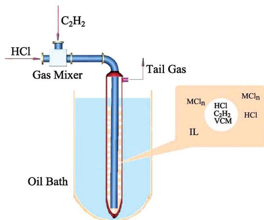
**Fig. 1** Reactor illustration for a gas-liquid acetylene hydrochlorination.
