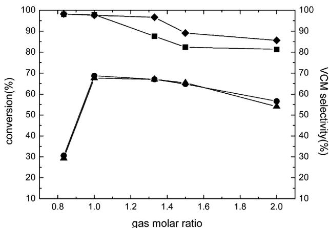
**Fig. 4** Influence of HCl/C<sub>2</sub>H<sub>2</sub> molar ratio on acetylene hydrochlorination in [Bmim]Cl (● acetylene conversion, ◆ VCM selectivity, 160 °C, CuCl<sub>2</sub>: 0.319 mol L<sup>-1</sup>; ▲ acetylene conversion, ■ VCM selectivity, 180 °C, CuCl<sub>2</sub>: 0.664 mol L<sup>-1</sup>).
