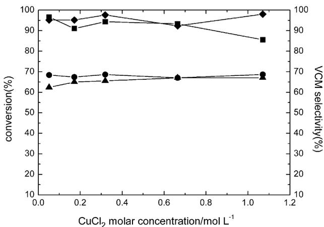
**Fig. 6** Influence of CuCl<sub>2</sub> concentration on acetylene hydrochlorination in [Bmim]Cl (● acetylene conversion, ◆ VCM selectivity, 160 °C, HCl: 0.31 L h<sup>-1</sup>; C<sub>2</sub>H<sub>2</sub>: 0.3 L h<sup>-1</sup>; ▲ acetylene conversion, ■ VCM selectivity, 140 °C, HCl: 0.4 L h<sup>-1</sup>; C<sub>2</sub>H<sub>2</sub>: 0.3 L h<sup>-1</sup>).
