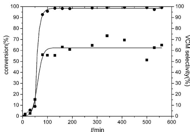
**Fig. 8** Influence of running time on acetylene hydrochlorination in [Bmim]Cl (■ acetylene conversion, ● VCM selectivity. 140 °C, HCl: 0.4 L h<sup>-1</sup>; C<sub>2</sub>H<sub>2</sub>: 0.3 L h<sup>-1</sup>; CuCl<sub>2</sub>: 0.058 mol L<sup>-1</sup>).
