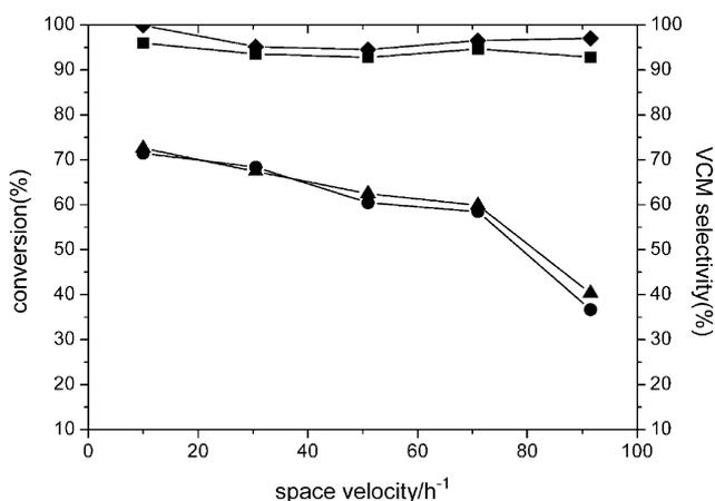
**Fig. 5** Influence of space velocity on acetylene hydrochlorination in [Bmim]Cl (● acetylene conversion, ◆ VCM selectivity, 160 °C, CuCl<sub>2</sub>: 0.051 mol L<sup>-1</sup>; ▲ acetylene conversion, ■ VCM selectivity, 180 °C, CuCl<sub>2</sub>: 0.172 mol L<sup>-1</sup>).
