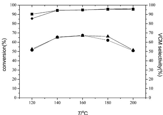
**Fig. 7** Influence of temperature on acetylene hydrochlorination in [Bmim]Cl (● acetylene conversion, ◆ VCM selectivity, HCl: 0.31 L h<sup>-1</sup>; C<sub>2</sub>H<sub>2</sub>: 0.3 L h<sup>-1</sup>; CuCl<sub>2</sub>: 0.051 mol L<sup>-1</sup>; ▲ acetylene conversion, ■ VCM selectivity, HCl: 0.4 L h<sup>-1</sup>; C<sub>2</sub>H<sub>2</sub>: 0.3 L h<sup>-1</sup>; CuCl<sub>2</sub>: 0.319 mol L<sup>-1</sup>).
