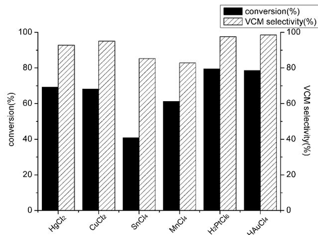
**Fig. 3** Different metal chlorides as catalyst for acetylene hydrochlorination (reaction conditions: IL: [Bmim]Cl; 160 °C; C<sub>2</sub>H<sub>2</sub>: 0.3 L h<sup>-1</sup>; HCl: 0.31 L h<sup>-1</sup>; catalyst concentration: 0.069 mol L<sup>-1</sup>).
