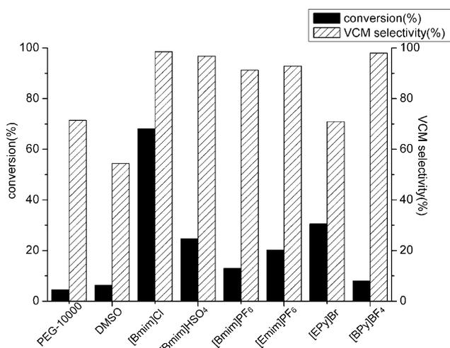
**Fig. 2** Acetylene hydrochlorination in different liquid media using CuCl<sub>2</sub> as catalyst (reaction conditions: 160 °C; HCl: 0.4 L h<sup>-1</sup>; C<sub>2</sub>H<sub>2</sub>: 0.3 L h<sup>-1</sup>; CuCl<sub>2</sub>: 0.058 mol L<sup>-1</sup>).
