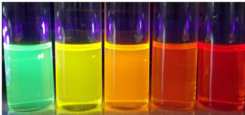
Fig. 4. Fluorescence solvatochromism of dye **4** in organic solvents. From left to right:  $n$ -hexane, benzene, chloroform, acetone and dimethylsulfoxide.
