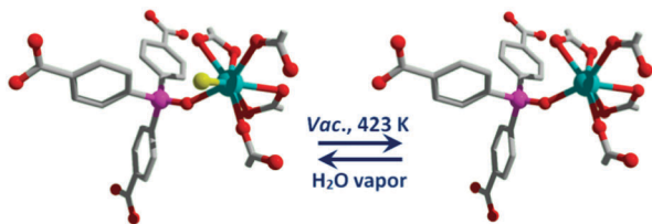
Scheme 1 Left: expanded view of the asymmetric unit in as-synthesized PCM-15; right: after removal of the single OH 2 ligand from the Tb(III) coordination sphere. Tb = cyan; P = magenta; OH 2 = yellow.
