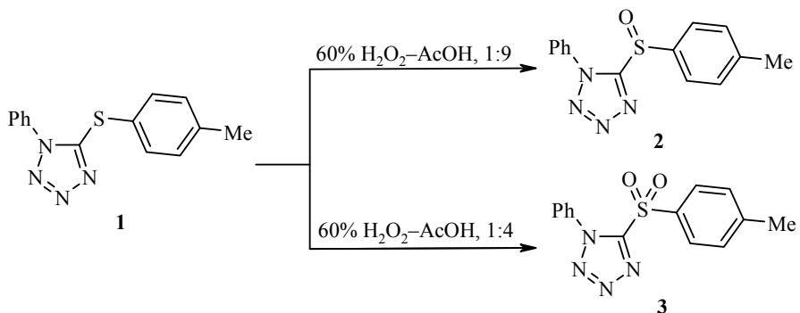
Oxidation duration on convection heating of compound **1** to compound **2** is 3 h. In the course of the reaction yet before full conversion of compound **1**, the product of full oxidation **3** begins to accumulate in the reaction mixture, that leads to a lowering of the yield and the need to use chromatographic methods for the
