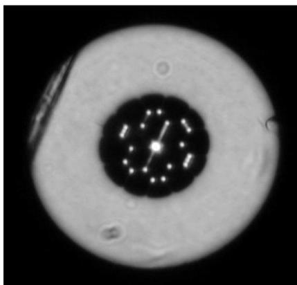
Figure 3. Optical micrograph of the output face of a fiber similar in size to that shown in Figure 2, illuminated with a white-light source at the far end. In addition to the core-guided modes, there are relatively weakly guided modes trapped at specific locations in the cladding, as well as confined modes, which include the core and a part of the cladding. Such modes become more strongly guided as the scale of the fiber is increased.
