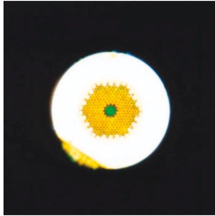
*Figure 4. Optical micrograph of the output face of an air-core photonic-bandgap fiber illuminated at the input face using a white-light source. The core is surrounded by the photonic-crystal cladding, which is embedded within a pure silica jacket. The air core has an area of seven unit cells. The strongly colored light in the core is confined by the bandgap of the surrounding photonic crystal. The outer diameter of the fiber is 110  $\mu\text{m}$ .*
