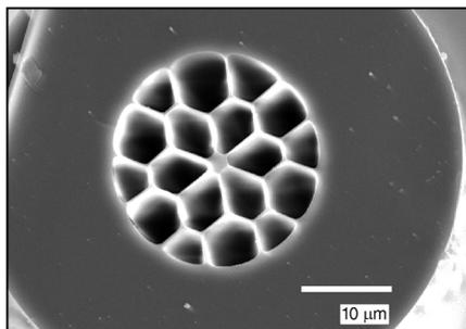
Figure 2. Scanning electron micrograph of a high-index-contrast total-internal-reflection-guiding PCF. The 2- $\mu\text{m}$ -diameter core is suspended in a web of 200-nm-wide silica strands, which are continuous along the fiber length.
