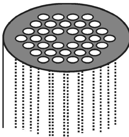
Figure 1. Schematic illustration of a "photonic-crystal fiber" (PCF). A fine silica fiber has a two-dimensional array of airholes running down its length. This photonic-crystal material can then be used to trap light in a core region. In the case shown here, the core is defined by a missing airhole in the center of the array.
