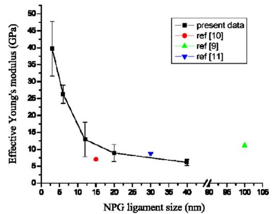
FIG. 2. (Color online) Plot of effective Young’s modulus of nanoporous gold leaf as a function of ligament size. The modulus in GPa is plotted on the y axis and ligament size in nanometers on the x axis; error bars mark one standard deviation in the data. Data points for 100 and 15 nm ligament NPG from Refs. 9 and 10 are also marked.
