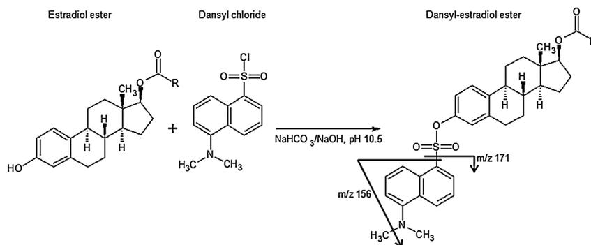
**Figure 2.** Scheme of dansyl chloride derivatisation reaction on estradiol esters (R is an alkyl group) and illustration of the MS fragmentation of the protonated dansyl-estradiol ester with the resulting two product ions.
