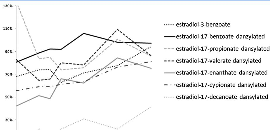
**Figure 5.** Recoveries of dansylation for six estradiol-17-esters derivatised at 60 °C with a contact time from 0 to 60 min (three replicates per point). Estradiol-3-benzoate was introduced as non-reactive analyte.
