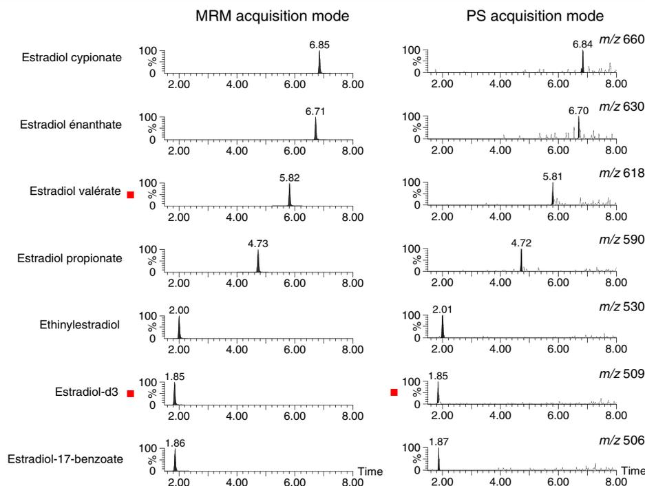
**Figure 6.** MRM (left) versus PS extracted chromatogram (right) using the Xevo TQMS mass spectrometer for estradiol-17-esters, estradiol-d3 and ethinylestradiol (0.2 ng injected).
