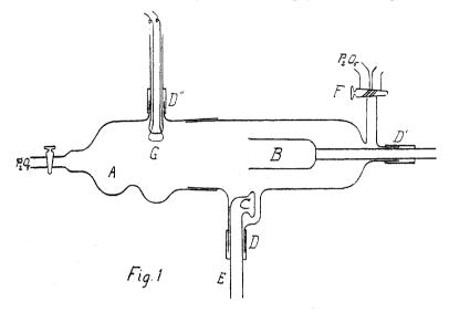
to obtain an atmosphere dry enough to make the transfer without hydrolysis. In order to detect possible hydrolysis after the transfer had been made, the two-way stopcock F was turned and the air within the apparatus was run into a solution of silver nitrate.
